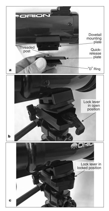
Figure 6. a) Attach the quick-release plate to the dovetail mounting plate on the telescope. b) Slide the quick-release plate into the pan head's saddle by tilting it and then pressing downward. c) Finally, close the lock lever to secure the telescope on the pan head.
