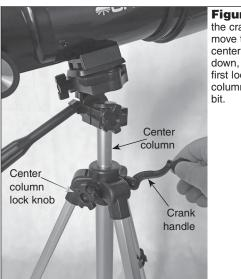
Figure 13. Use the crank handle to move the geared center column up or down, making sure to first loosen the center column lock knob a bit
