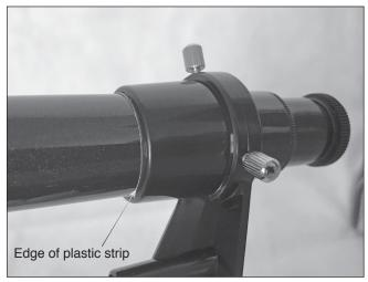
**Figure 8.** Slide the finder scope tube, eyepiece end first, into the bracket, making sure the plastic strip surrounds the tube. The strip should be just barely visible when the finder scope is fully inserted, as shown.
