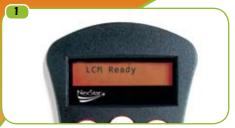
Turn power switch (located on the side of the base) to "on" position. The light will come on and the hand control will display "LCM Ready".
