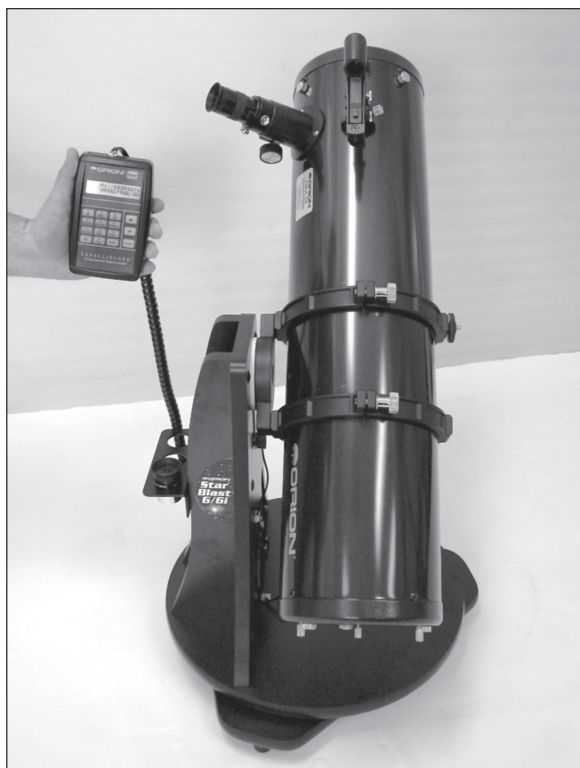
Figure 25. If you're positioned to the left of the telescope and face the direction the optical tube is pointed, the guide arrows on the Computerized Object Locator will correspond exactly with the direction you should move the telescope to pinpoint the selected object.
