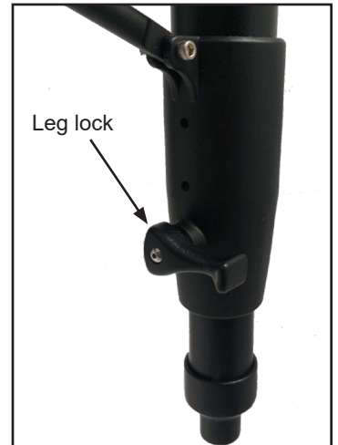
Fig. 7: Loosen lock lever, extend inner leg, relock lever.
