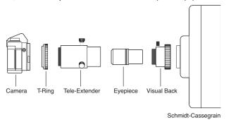
C-90s and some other small spotting scopes have threads that will fit a tele-extender directly but require the use of .965" eyepieces to create the higher magnifications.)
