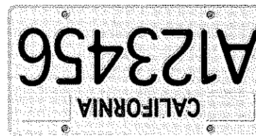
Figure 11. The view through a standard finder scope and reflector telescope is upside down. This is true for the SkyQuest XT4.5 and its finder scope as well.
