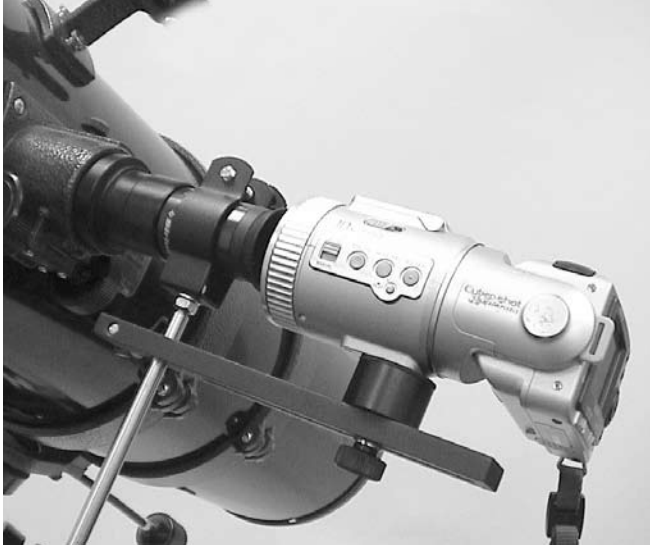
Figure 3. By orienting the camera and SteadyPix assembly as shown you will bring the center of mass of the assembly as low as it can get. This will prevent the SteadyPix and camera from rotating downward.
