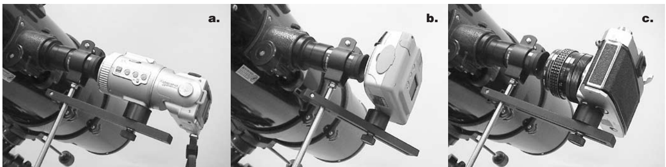
Figure 6. The same cameras in Figure 5, but with the SteadyPix attached to a telescope and ready to shoot. Note how the camera support plate must be adjusted for different camera designs.
