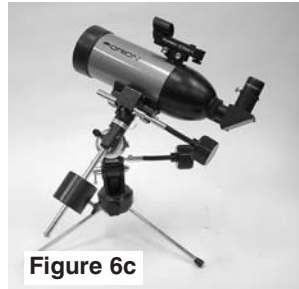
Figure 6a,b,c,d. This illustration shows the telescope pointed in the four cardinal directions: (a) North, (b) South, (c) East, (d) West. Note that the tripod and mount have not been moved; only the telescope tube has been moved on the R.A. and Dec. axes.
