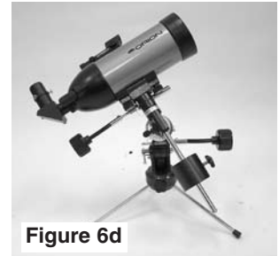
Figure 6a,b,c,d. This illustration shows the telescope pointed in the four cardinal directions: (a) North, (b) South, (c) East, (d) West. Note that the tripod and mount have not been moved; only the telescope tube has been moved on the R.A. and Dec. axes.
