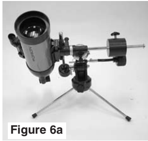
Figure 6a,b,c,d. This illustration shows the telescope pointed in the four cardinal directions: (a) North, (b) South, (c) East, (d) West. Note that the tripod and mount have not been moved; only the telescope tube has been moved on the R.A. and Dec. axes.
