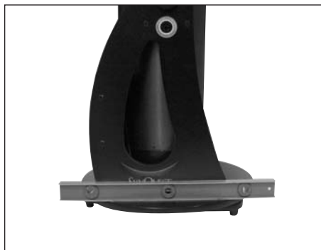
Figure 7. Place a carpenter's level on the base as shown. The base should stay level through a 180° rotation in azimuth. Once the vertical stop is set, the base does not need to be level to function properly.
