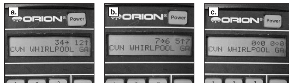
Figure 10a-c. This sequence of pictures illustrate how the controller’s guide arrows will look as you are finding an object. (a.) When you are far away from the object, there will be a number (from 10 to 179) to the left of the guide arrows. (b.) When you are close to the object, each guide arrow will display a number on its immediate left (from 0 to 9) and immediate right (from 0 to 9); the number on the left is whole number increments, while the number on the right is in increments of tenths. This helps in making small movements to the telescope to pinpoint the object’s location. (c.) When the guide arrows display “0.0 0.0”, the object will be within the field of view of the telescope (with a 25mm or longer focal length eyepiece).
