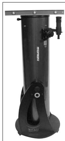
Figure 8. Once the base is leveled, point the tube up until the mirror cell comes into contact with the vertical stop. Then, place the carpenter's level across the top of the tube as shown. If the vertical stop is set properly, the top of the tube should also be level.
