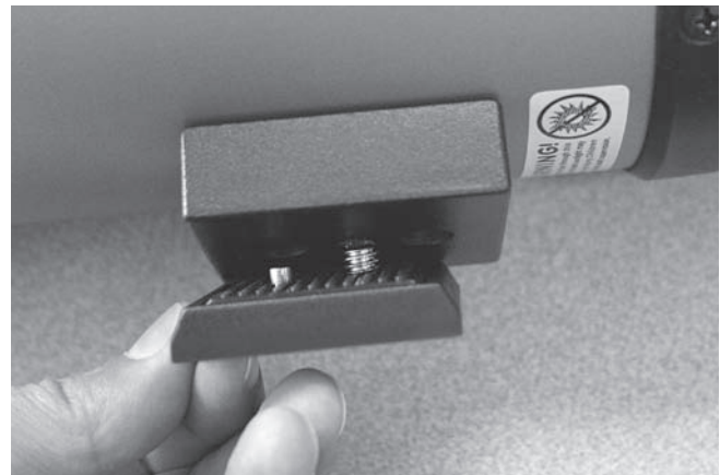
Figure 2b. Orient the quick-release shoe relative to the mounting block as shown.
