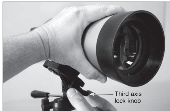
Figure 6. The tripod's third axis of motion is rarely, if ever, used.
