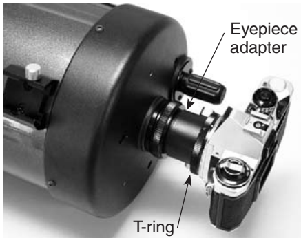
Figure 2. A T-ring is all that is needed to connect a 35mm SLR camera to the telescope; it threads onto the eyepiece adapter with eyepiece and diagonal removed.
