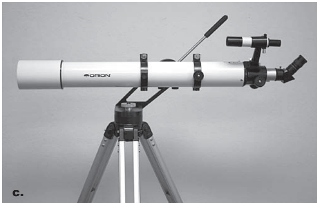
Figures 15a-c: The telescope is not balanced because it is front-heavy. (b.) The telescope is too back-heavy. (c.) The telescope is properly balanced on the altitude axis.
