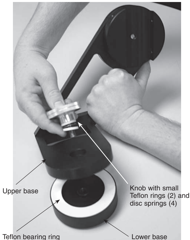
Figure 9. Position the upper base over the lower base, and connect the parts by passing the knob through the upper base and threading it into the lower base. The Teflon bearing ring should seat between these parts.
