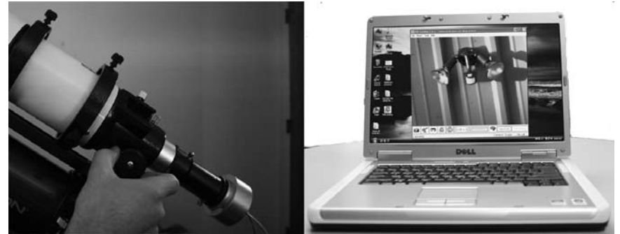
Figure 8. Gradually move the focuser inward until you have a clear daytime image on your computer screen.
