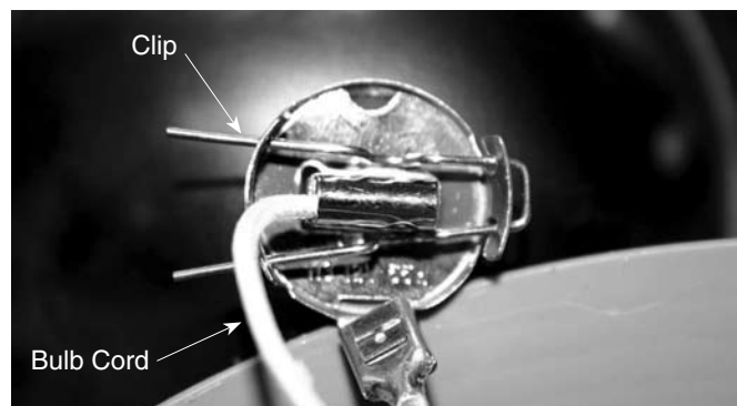
Figure 2. Remove the clip to separate the bulb assembly from the reflector.
