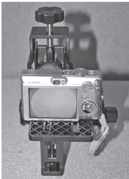
Figure 2. Camera position relative to the telescope eyepiece should be adjusted until the image covers as much of the LCD screen as possible.
