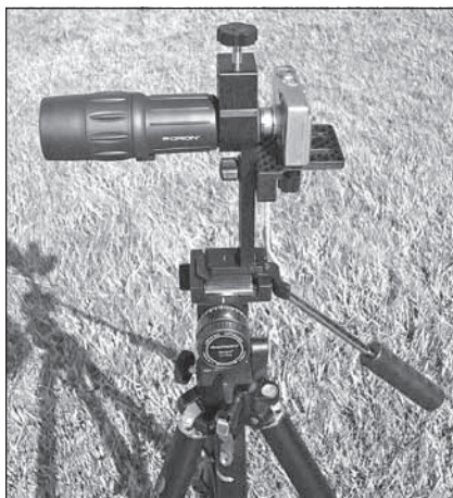
Figure 4. The Orion Digiscoping Adapter is shown attached to a photo tripod via the 1/4"-20 socket in the adapter's foot. A monocular is held in the eyepiece clamp.
