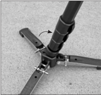
Figure 4. Rotate the knurled tilt adjustment ring near the bottom of the monopod up or down to allow a greater or lesser amount of tilt, respectively. Allowing more tilt can be useful when photographing or observing moving subjects
